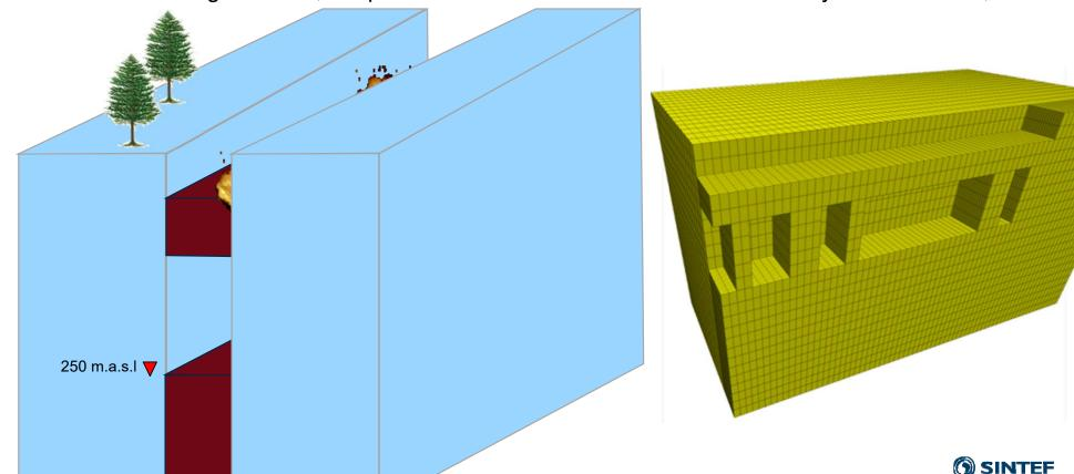
After removing the pillar, the mine will be developed in 4 mining levels: 221; 187; 153; 123
