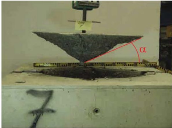
Figure 2.5: An example of a cone failure in concrete. From Nilsson and Elfgrén (2009)
