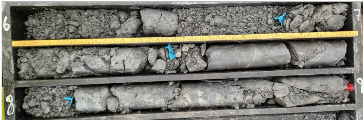
Figure 2: Sandy/gravelly material alternating with clayey material and shear bodies (KP2b_Oct24, 6-9 m).
