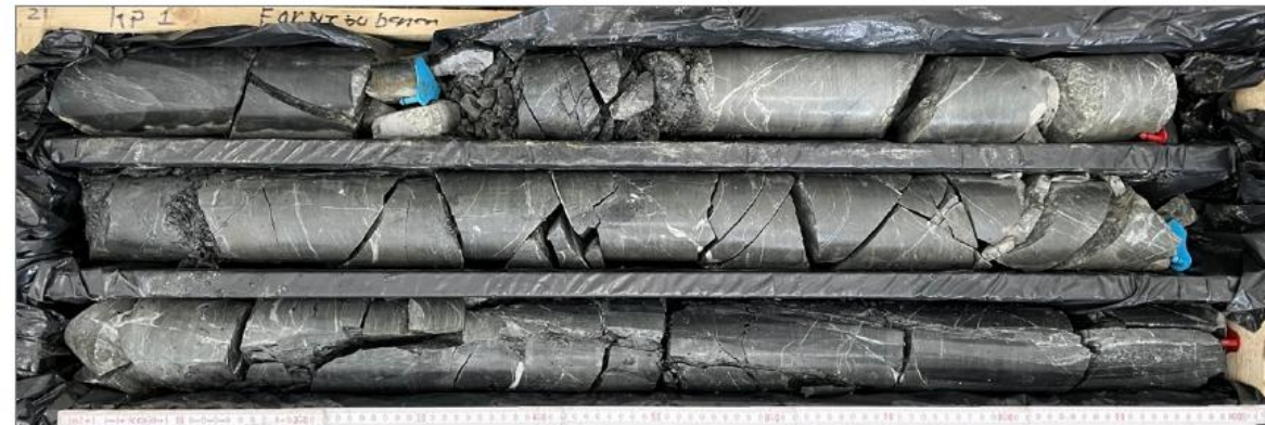
Figure 5: Fractured but otherwise undisturbed rock mass of the damage zone (KP1_Sep24, 21-24 m).
